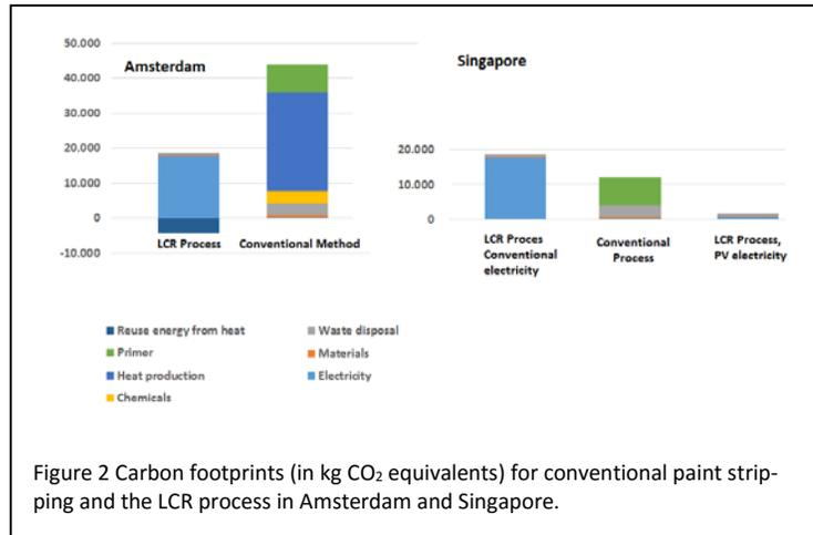
Figure 2 Carbon footprints (in kg CO<sub>2</sub> equivalents) for conventional paint stripping and the LCR process in Amsterdam and Singapore.
